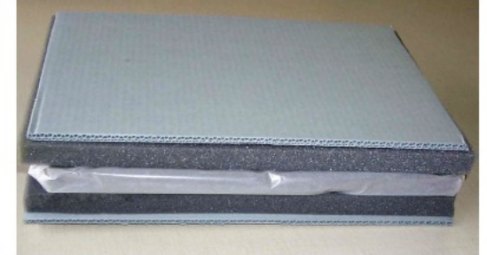
Figure 4. Sandwich the foam package between two layers of multi-use corrugated board.
