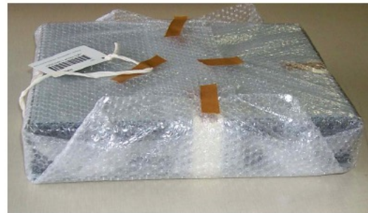
Figure 6. Tape an identification tag on top of the bubble wrap.
