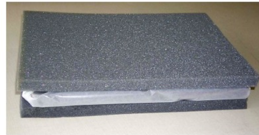
Figure 3. Sandwich the glassine-wrapped frame between urethane foam.
